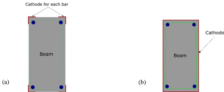
Figure 4. Cathode position (a)  $C_1$  configuration (b)  $C_2$  and  $C_3$  configurations.
