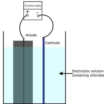
Figure 1. Set-up for accelerated corrosion by imposed current.
