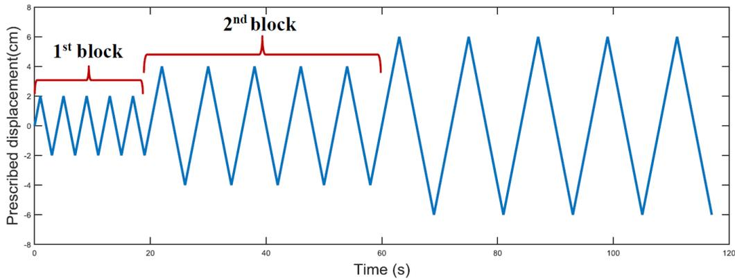
Figure 7. Planned load in quasi-static testing.
