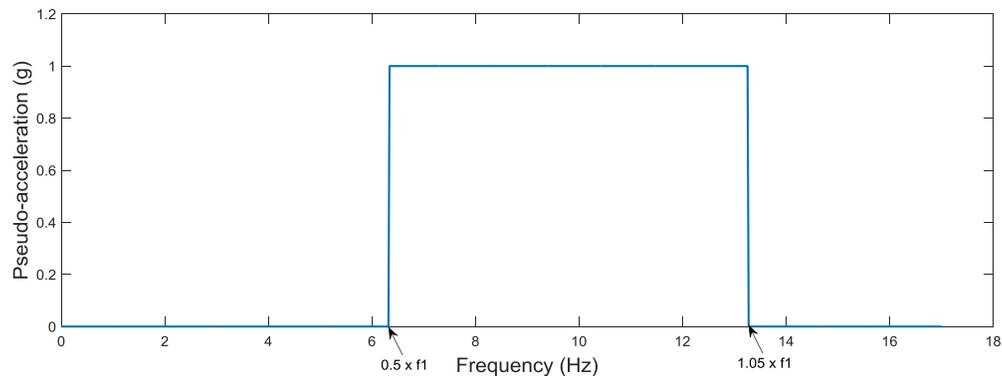
Figure 9. Crenel spectrum used in signal generation.
