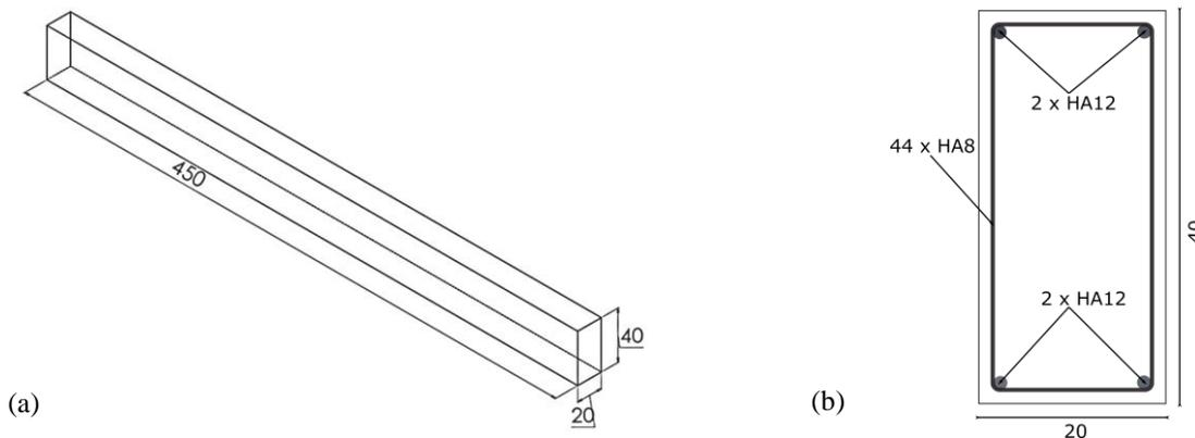
Figure 3. Specimen's design: (a) Geometry, (b) Reinforcement details. - dimensions in centimeters-
